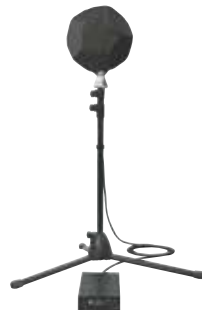
Miniature dodecahedron speaker for room acoustic measurements
